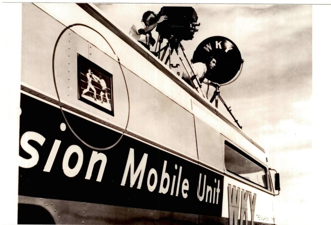
Figure 7. Microwave remote television production truck. Circa 1949. Notice 155 sq. inch television receiver built into side of production truck. Camera and microwave transmission dish on truck's roof.
