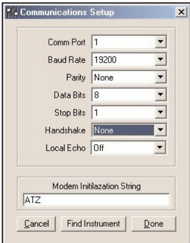
After modifying the EasySpan CommPort table above, the instrument's RS-232 settings must be modified to reflect the same settings. After matching up the settings **[Click]** on **[Find Instrument]** and the PC should find the instrument and display its model and serial number on the screen. If it doesn't, check the settings and cable to make sure they are correct.
